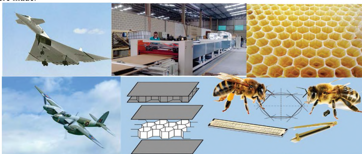
Figure 11: Manufacture of honeycombs by bees, humans and their application in honeycomb panels on airplanes Mosquito and B-58
