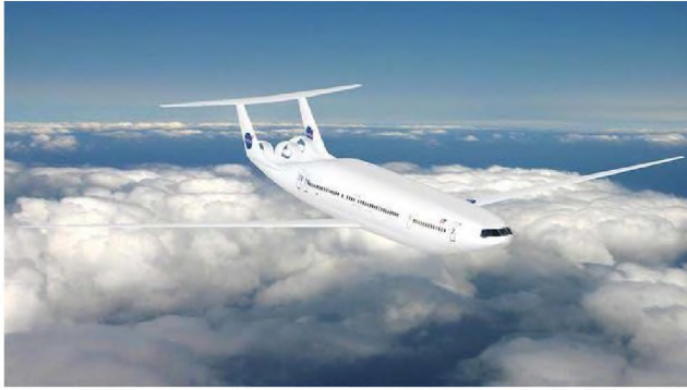
Figure 6: MIT Double-bubble Fuselage with Aft-mounted engines
