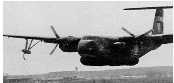
b) Aircraft with ACLG DHC-5/CC-115«Buffalo» (Bell Aerospace 1971/USAF 1975-79 Canada, USA)
