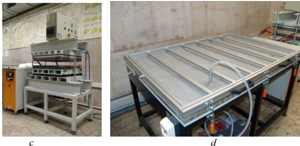
Figure 8 ( cont'd ): Equipment for Thermal Compression Molding: a – Autoclave; b – Hydraulic Press; c – Pneumatic Press; d – Vacuum Press.
