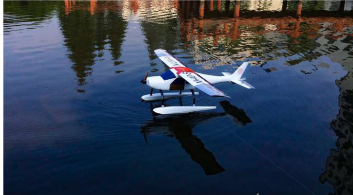
Figure 6: Taxi test of the EPUAV on the lake at NUAA campus
