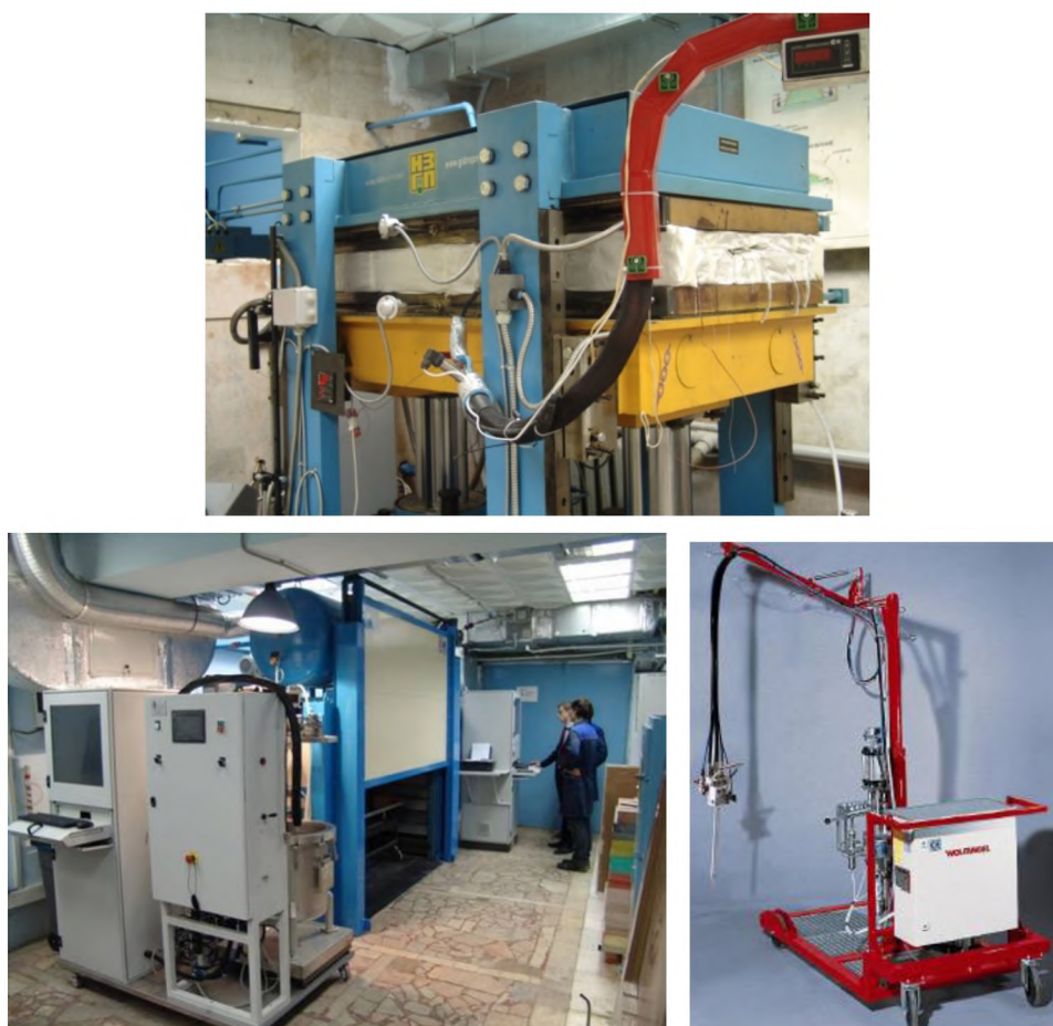
Figure 8 ( cont'd ): Equipment for Thermal Compression Molding: a – Autoclave; b – Hydraulic Press; c – Pneumatic Press; d – Vacuum Press.
